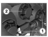
Remove the covers 1 on the high-beam bulbs and/or the cover 2 on the low-beam bulbs by turning counterclockwise.
